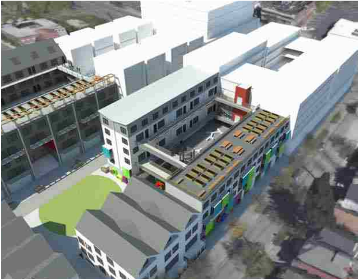
Fig. 4.68 Site C: birdseye perspective facing northwest from 24th and Spring. Circulation is provided via external walkways allowing units to exit directly into the open air. The second floor central courtyard occupies a portion of the central open space and provides shared private open space for residents. The southern half of this void is at grade and accommodates a dedicated outdoor play space for the ground floor day care facility. The roof terrace allows residents to grow food and provides views of the Cascades.
